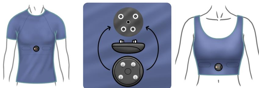
Snap the Oxa sensor into the front of the garment. Locate the contacts and insert the sensor so that all the pins are connected properly.
